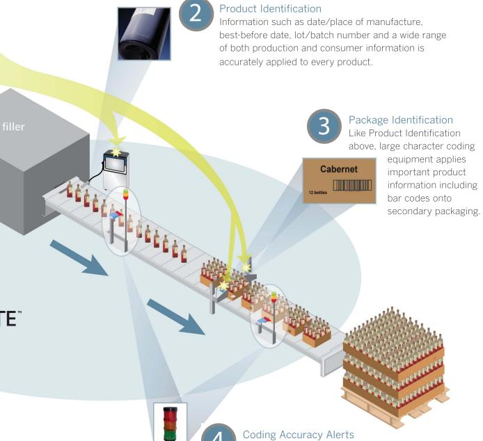
Throughout the packaging line, scanners check codes for accuracy. If a coding accuracy issue is detected, the alarm beacon can be activated and the line can be stopped or the product rejected automatically.
