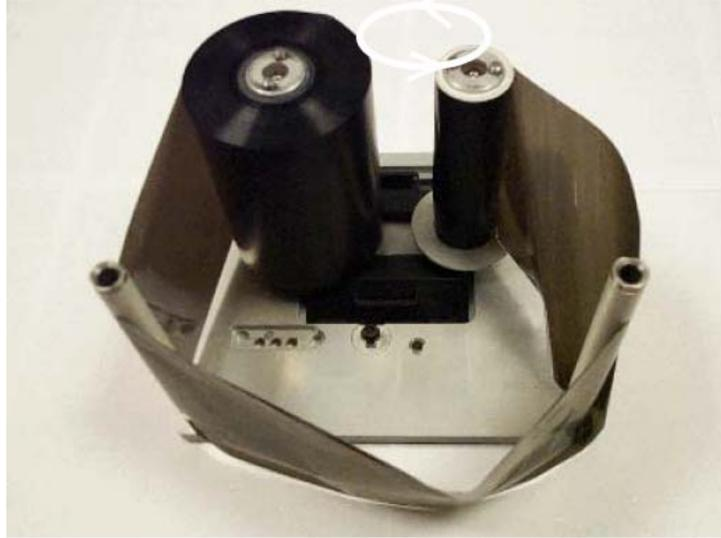
Figure 5-13: Ribbon Spool Routing
