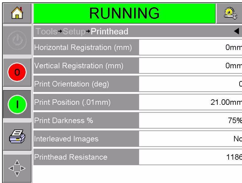
Figure 4-13: Printhead Setup Page for Continuous Motion Applications
