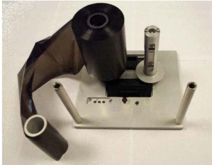
*Figure 5-12: Ribbon Spool Installation*
