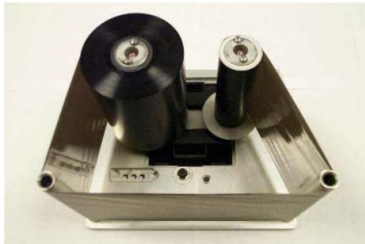
Figure 5-14: Ribbon Spool Routing
