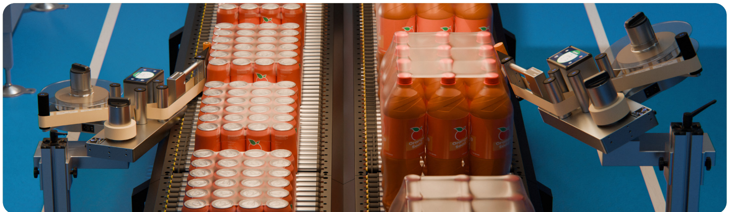
Dual lane, side application configuration
