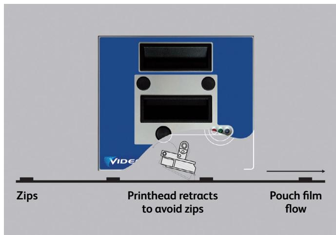
**A simple software setting can retract the thermal transfer printhead up to 4.5mm**
