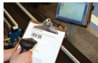
Job data can be sent to the printer via a hand-held scanner
