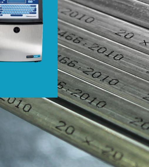
**The company's current printing requirements consist of their company brand and logo, date, lot number, type of product and the quality standard onto the fabricated steel products. Coding each product with this level of detail helps Chinh Dai to meet retailer regulations and government requirements, as well as promoting their own brand.**
