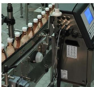
Some of Ultra Dairy's bottled products require a code the company uses for tracking purposes. This code enables Ultra Dairy to keep unique information about the bottling process right on the bottle, including information about the fill head, foil head and cap head involved in the bottling process. Since this code is only used by Ultra Dairy and is covered by a sleeve, the company wanted to make sure the code wasn't visible through the sleeve.
